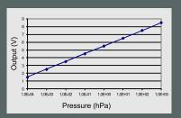
$V_{out}(V) = log(p(hPa)) + 5.5$  $p (hPa) = 10^{(V_{Out}(V) - 5.5)}$
