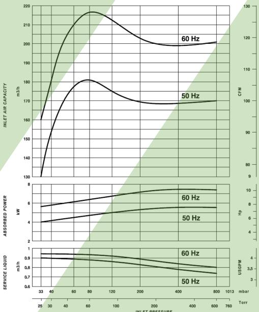
The given data are referred to dry air at the temperature of 20°C, at the atmospheric discharge pressure (1013 mbar), and of supply of service water at 15°C temperature. Performances tolerance ±10%.
